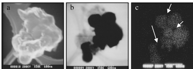
Figure 2. (a) SEM, (b) STEM images and (c) corresponding EDS elemental map for Fe of \text{LiFePO}_4 observed by TEM.
